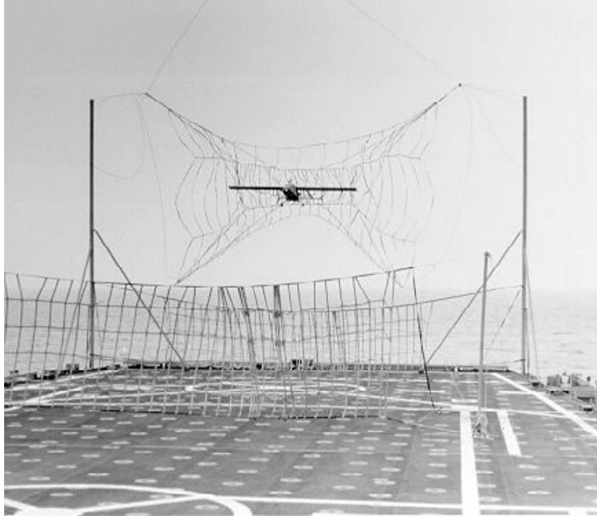
Fig. 15 - Shipboard landing of the Pioneer into the capture net while being flown remotely by a pilot on ship deck (actual photo).
