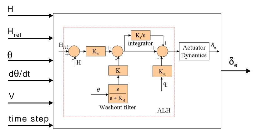
Airspeed V is used to set the gains.
