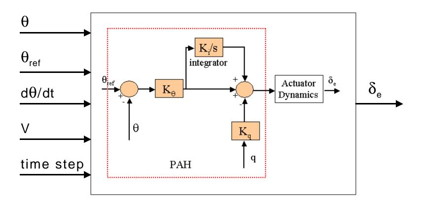
Airspeed V is used to set the gains.
